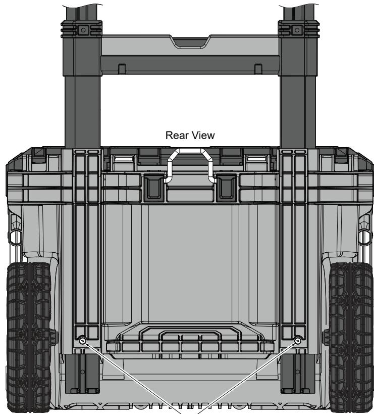
Locking Casters (1) are to be assembled to the front of the PACKOUT™ Dolly Body (3). Front of the dolly body is determined by the logo plate.
