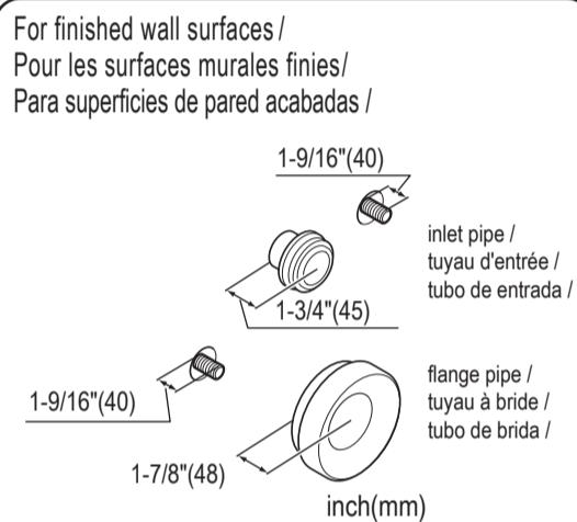
**EN** **WARNING:** Installation surface must be completely flat and on plane. Uneven surfaces can cause bowl to crack or break.
