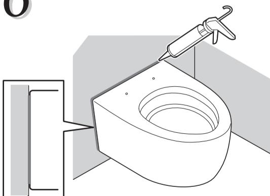
When installing the washlet main unit or standard toilet seat main unit, follow the instructions in the included Installation Guide.
