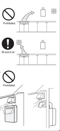
State of California: The water heater must be braced, anchored or strapped to avoid moving during an earthquake. Contact local utilities for code requirements in your area or call: 1-866-766-7489 and request instructions.
