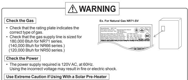
• Using this unit with a solar pre-heater can lead to unpredictable output temperatures and possibly scalding. If absolutely necessary, use mixing valves to ensure output temperatures do not get to scalding levels.
