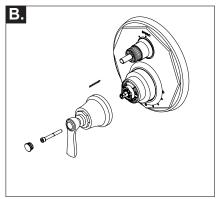
Models with axial screw in handle blade -Secure handle onto the stem using screw and hex wrench or screwdriver as needed. Insert button into handle.
