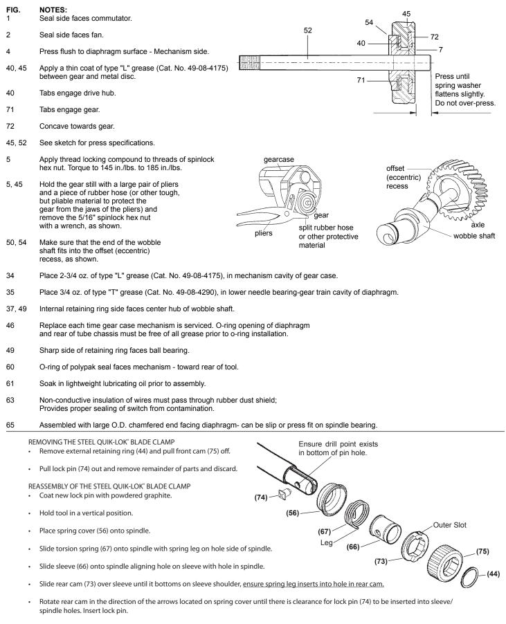
Align front cam (75) inner ribs with rear cam outer slots and slide front cam onto sleeve until it bottoms. Retaining ring (44) groove should be completely visible.
