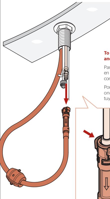
**To remove Hose, press on the Tabs and pull Hose Connector down.**
