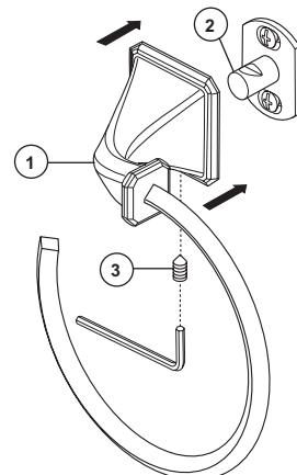
Position body (1) over mounting stud (2) and tighten set screw (3).
