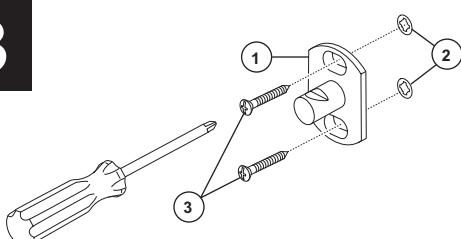
With the mounting stud (1) oriented as shown, place it over the installed anchors (2) and install screws (3).
