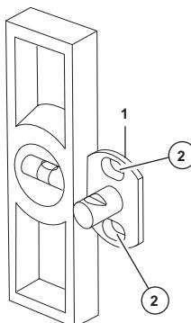
**NOTE:** If possible, it is best to mount your accessory into a wall stud. Try to locate a wall stud with a stud finder or by tapping on the wall. Place mounting stud (1) in the desired location. Ensure the mounting stud is level; then, mark the position of the holes (2) on the wall.
