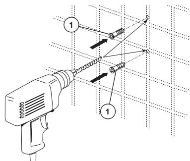
If you were able to locate a wall stud to mount your accessory or if you are mounting it to a door, drill 1/8" (3mm) holes and mount the mounting stud with the two #8 screws provided. (Skip to step 4).
