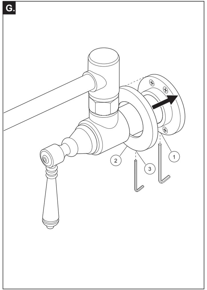
**E.** Wrap plumber tape (1) around pipe threads. Install the gasket (2) and the flange (3) using the 4 screws (and anchors if required) provided.
