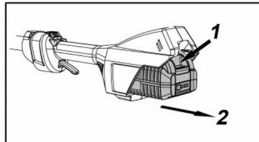
**CAUTION:** Protect the battery contacts when the battery is not being used. Loose metal parts may short-circuit the contacts – **Explosion and fire hazard!**
