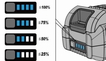
The indicator goes out after 3 seconds. If one of the LEDs flashes, the battery must be recharged. If none of the LEDs light up after the button is pressed, the battery is faulty and must be replaced.
