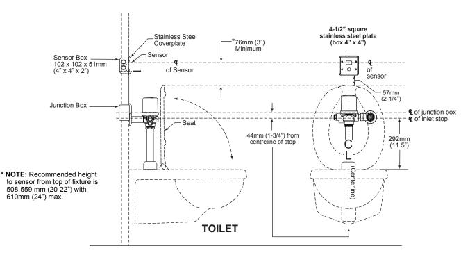
NOTE: Hardwire juction box installed behind flush valve on centerline of fixture.
