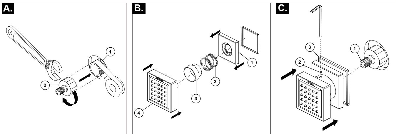
**A.** Apply plumber tape to the pipe nipple (1). Thread trim body (2) onto pipe nipple. Tighten securely with wrench.
