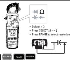
Range Resolution Accuracy **Overload Protection** 10.00nF 0.01nF 100.0nF 0.1nF 1.000uF 0.001uF 2.5% + 5dqts 600V RMS 10.00uF 0.01uF 100.0uF 0.1uF 9999uF 1uF 3.0% + 5dgts
