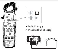
• Buzzer sounds at less than  $< 40\Omega$ .
