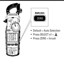
The UEi LRA Inrush is programmed to properly capture the starting current for compressor motors.
