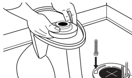
Carefully align and lower the toilet over and onto the closet flange while having the T-bolts come through the holes of the bowl. Firmly press down and apply weight evenly.
