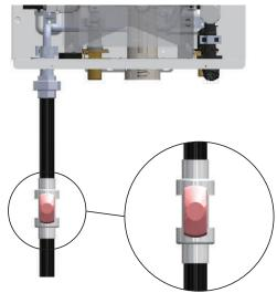
5. Check for a gas leak at the gas connection portion with soapy water.
