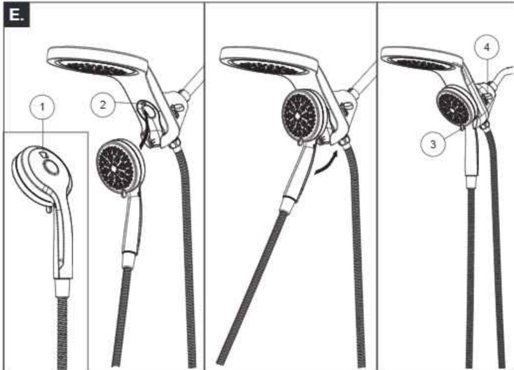
To combine the two showers, insert the top slot (1) on the hand shower into the tab (2) of the shower head. Push the hand shower into the shower head until the two parts snap together.
