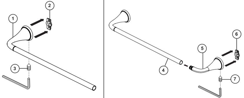
Position body (1) over mounting bracket (2) and tighten set screw (3). (Set screw should be on the bottom of body.) Place one end of the towel bar (4) into the second body (5), and place the other end of the bar into the first body (1). Slide the second body over the other mounting bracket (6) and tighten set screw (7).
