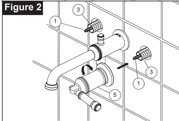
**NOTE: When drilling holes for hot and cold end valves, the hole size must be between 1 1/2" (38mm) and 1 5/8" (41mm).**
