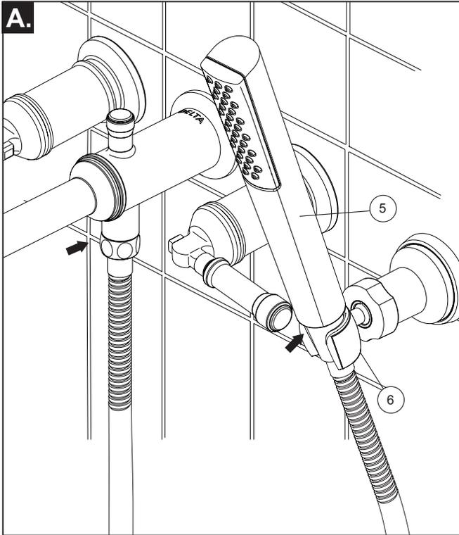
**A.** Turn on water supplies and hot & cold handles, check for leaks. Pull the diverter knob and check the leak between the connections. Check that the hand shower holder (6) can hold the handshower (5) in place. If not, tighten nut of holder.
