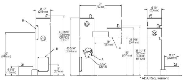
A = 3/8" O.D. Unplated copper tube connect
