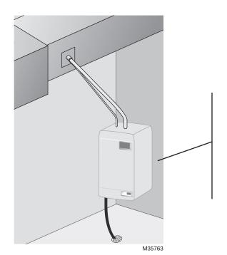
**Remote mounting.** The Electrode Steam is installed some distance away from your furnace supply duct. An insulated hose carries steam from the Electrode Steam to a suitable location on the supply duct.
