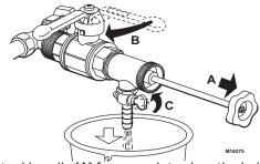
Pull out tool handle (A) far enough to clear the ball valve. Close off ball valve (B)
