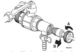
Unscrew end cap (A) and remove cartridge from chamber (B). Clean or replace cartridge as needed.
