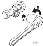
Remove T100 or T104 thermostatic control from radiator valve and loosen V100/V110 valve cartridge slightly (using MT110D1019 socket for V110 valves) (A and B)
