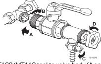
Tighten MT100/MT110 tool to valve body (A and B). Close shut-off cock (C) and turn tool counterclockwise to remove valve cartridge from the valve body (D)
