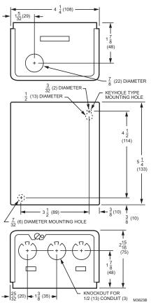
Fig. 1. R8845U dimensions in in. (mm).
