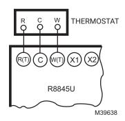
Fig. 8. R8845U thermostat connections.
