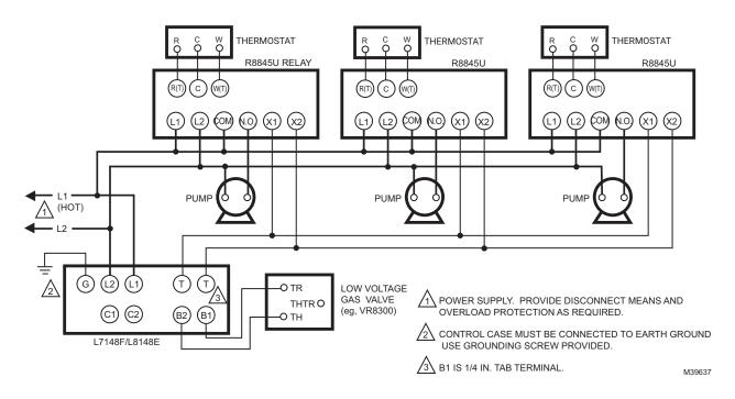
Fig. 6. R8845U hookup for L7148F/L8148E in a gas-fired, 24V, zoned, pump system.
