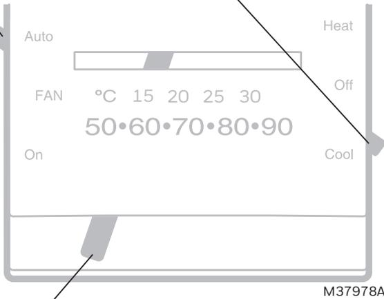
**Temperature setting:** Adjust to set desired indoor temperature.
