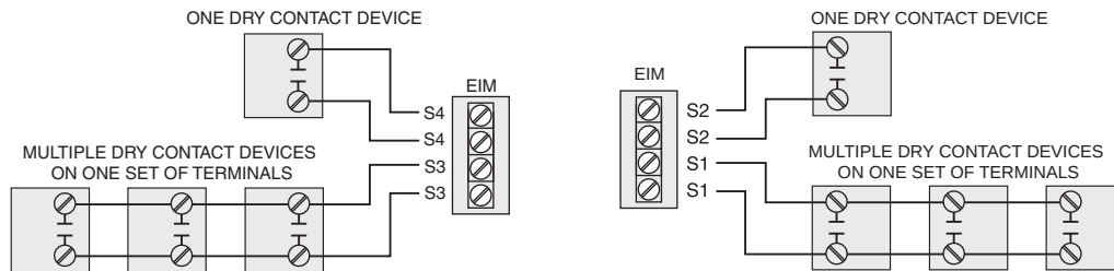
Fig. 157. Wiring dry contact devices.
