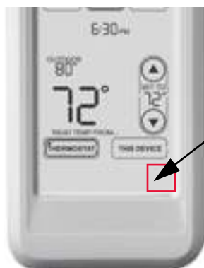
Fig. 48. Restarting the linking process.
