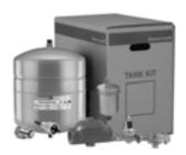
Honeywell TK Series Boiler Trim kits are a quick and convenient way to purchase the key "boiler trim" used by installers when performing a boiler change out. All Trim Kits with Purgers include expansion tank, air purger and air vent; selected models also include FM911 combination boiler fill valve / backflow preventer and/or service check valves for in-line servicing of the expansion tank and air vent.
