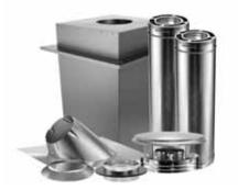
Kit includes: DVL and DuraBlack Adapter, 24" Square Ceiling Support Box with Trim, Adjustable Flashing 0/12-6/12, Chimney Cap, Storm Collar, and (2) 24" DuraPlus Chimney Pipe (galvanized). Only available in 6" diameter. Can be used for cathedral ceiling installations.
