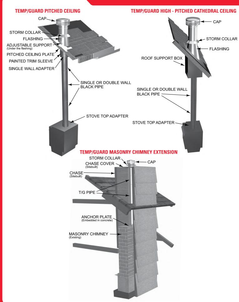
Note: Twist Lock Pipe (6"-12") overlaps  $1\frac{1}{2}$ " when joined together. Quick Connect Lock (14"-18") overlaps  $1\frac{1}{2}$ " when joined together with sheet metal screws. Therefore, assembled length on all sizes is  $1\frac{1}{2}$ " less than listed length.
