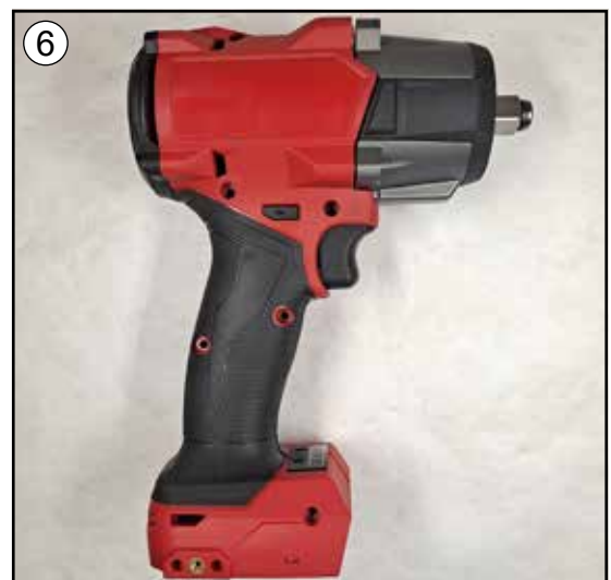
Install right handle half (cover) over left handle half (support). Check for the proper functionality of switch and shuttle. Secure handle halves together with seven screws.
