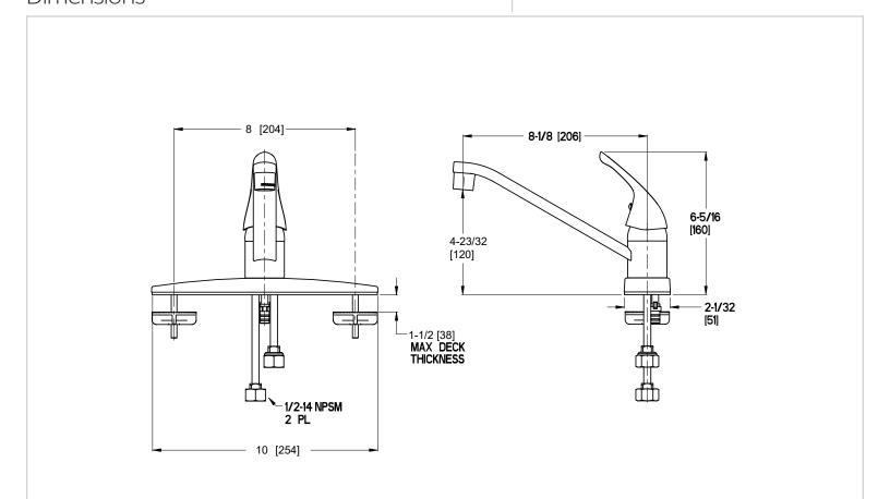
Ø1-3/8 Min to Ø1-1/2 Max. Deck Hole Openings
