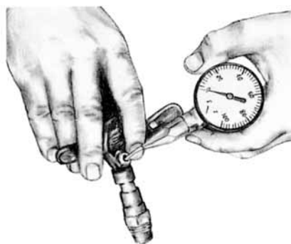
FIGURE 3 Pilot tube shown properly inserted into sprinkler nozzle. (Approx. 1/8" from nozzle opening)
