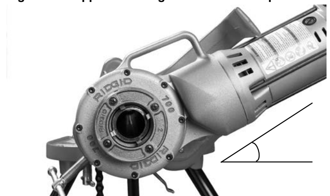
Figure 6 – Support Arm Positioned With 700 Power Drive Slightly Above Horizontal
