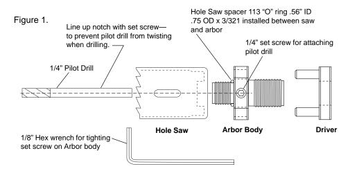
Note: Do not use pilot when drilling PVC pipe
