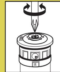
TO ADJUST RADIUS: Using a Phillips-head screwdriver, turn adjustment screw to right to decrease radius, to left to increase it.
