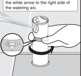
Turn the arc adjustment ring to align
